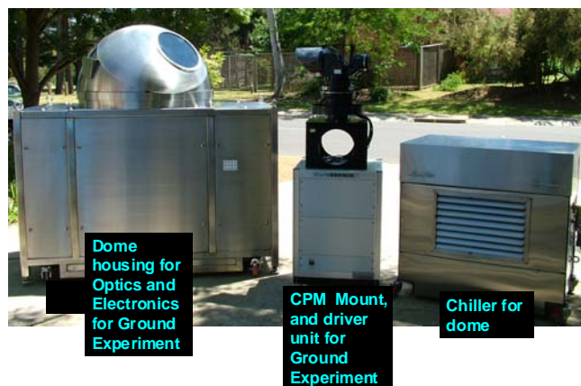
Figure 8: Utility development for Ground outside experiment
