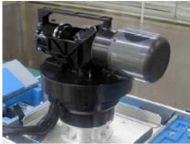
Figure 4: A 10cm class Coarse Pointing Mechanizm (CPM)
